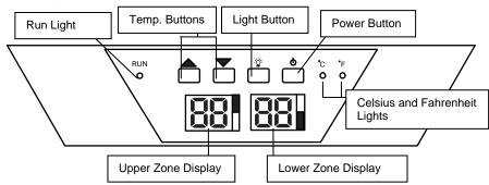
Use the up button to adjust the upper zone's temperature, and use the down button to adjust the lower zone's temperature. The temperature displayed can be in Fahrenheit or Celsius. This wine cooler has a temperature range from 41°F to 54°F for the upper zone, and 54°F to 64°F for the lower zone.
